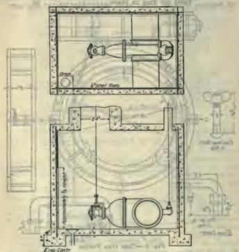
Fig. 9.—Concrete Vault for Horizontal Valve.
